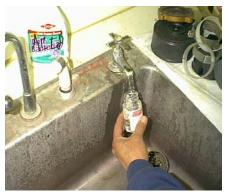
Grasp the container near the bottom (see picture above). NEVER touch the inside of the cap and the container.
