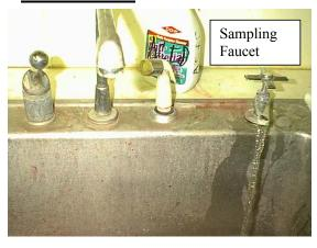
Indoor faucets in a clean area are the best sites for sampling. Make sure the faucet is not connected to a water softener, in-line filtration units, or hot water heater. These types of connections would not supply the water that is representative of the water in the distributions system. Avoid sampling from faucets that have swiveling heads, faucets with the hot and cold water under the same valve, or faucets with leaking valves.
