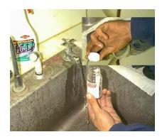
Do not set the container cap down! Hold it with fingers away from the edge and away from splashing water. DO NOT hold the lid upside down.
