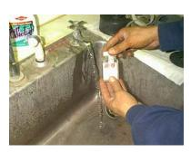
After the lines have been flushed, open the container. (The use of latex gloves will reduce the chance of contamination from the sampler.)
