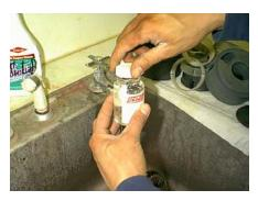
Affix the cap on the container as soon as it is filled and removed from the flow. Check to make sure that your container is properly sealed, as the sample will leak if not properly sealed.
